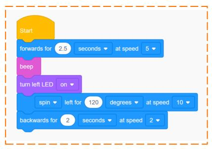
All EdScratch programs need to have the yellow Start block at the very top. This lets the robot know that the program starts with the first block below the Start block.
